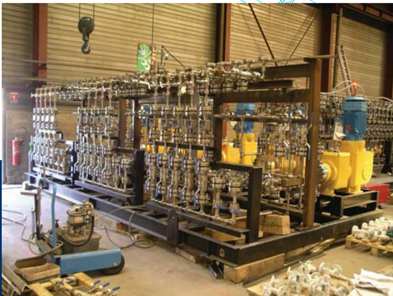
Set of trunnion mounted twin valves supplied for a skid of DALIA Project.
