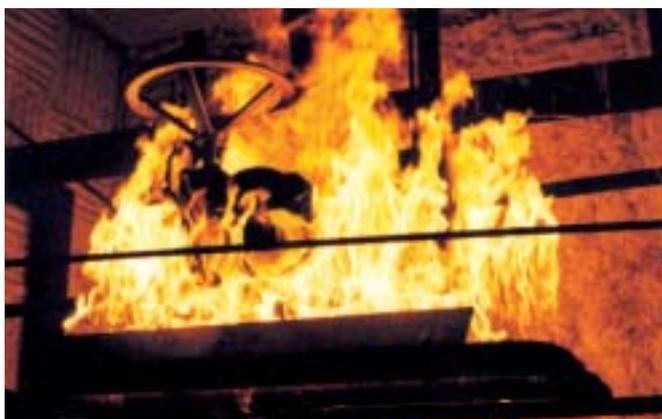
*Metal to Metal Seat, diaphragm sealing as well as the stem sealing compound with graphite guarantees a high reliability performance of our Plug Valves while in exposure to Fire Test conditions.*
