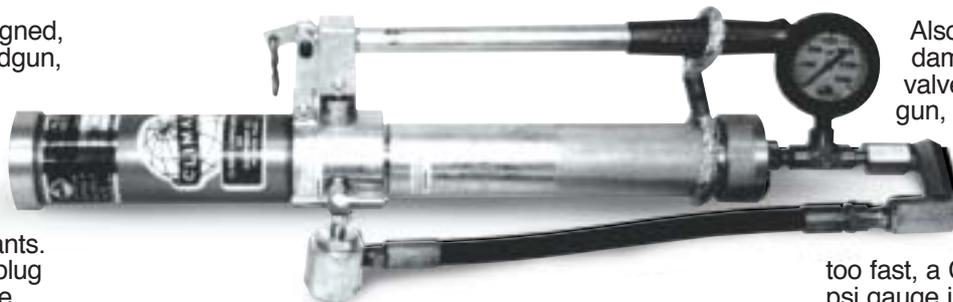
should it be opened tight against the stop. The valve should be closed firmly, but not tightly. It is not necessary to open the valve past one full turn. Due to "built - in" safety features, the CLIMAX 1699 provides the maximum
