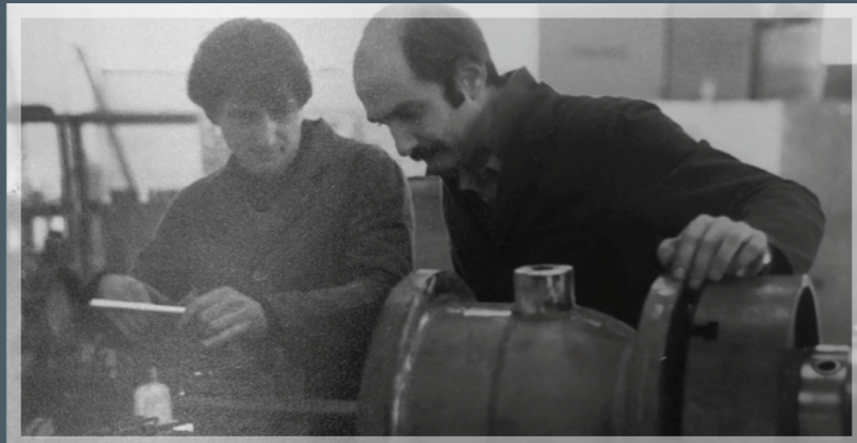
Valve machining with an horizontal lathe 1978
