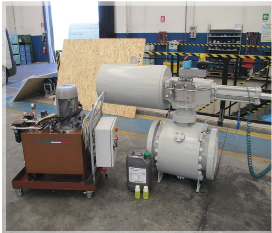
Actuator Flushing / NAS Cleaning
