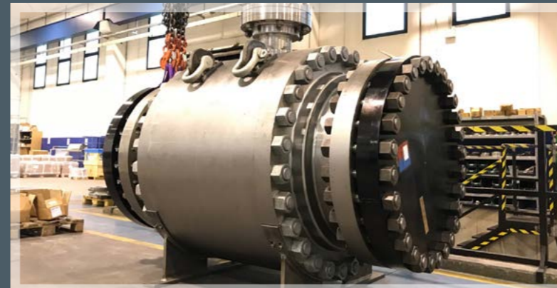
36" 600 class ball valves ready for test
